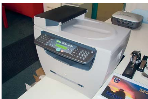
Tiskárna CANON MF5770-laserprint/copy/colScan/ fax/ADF-18 ppm
